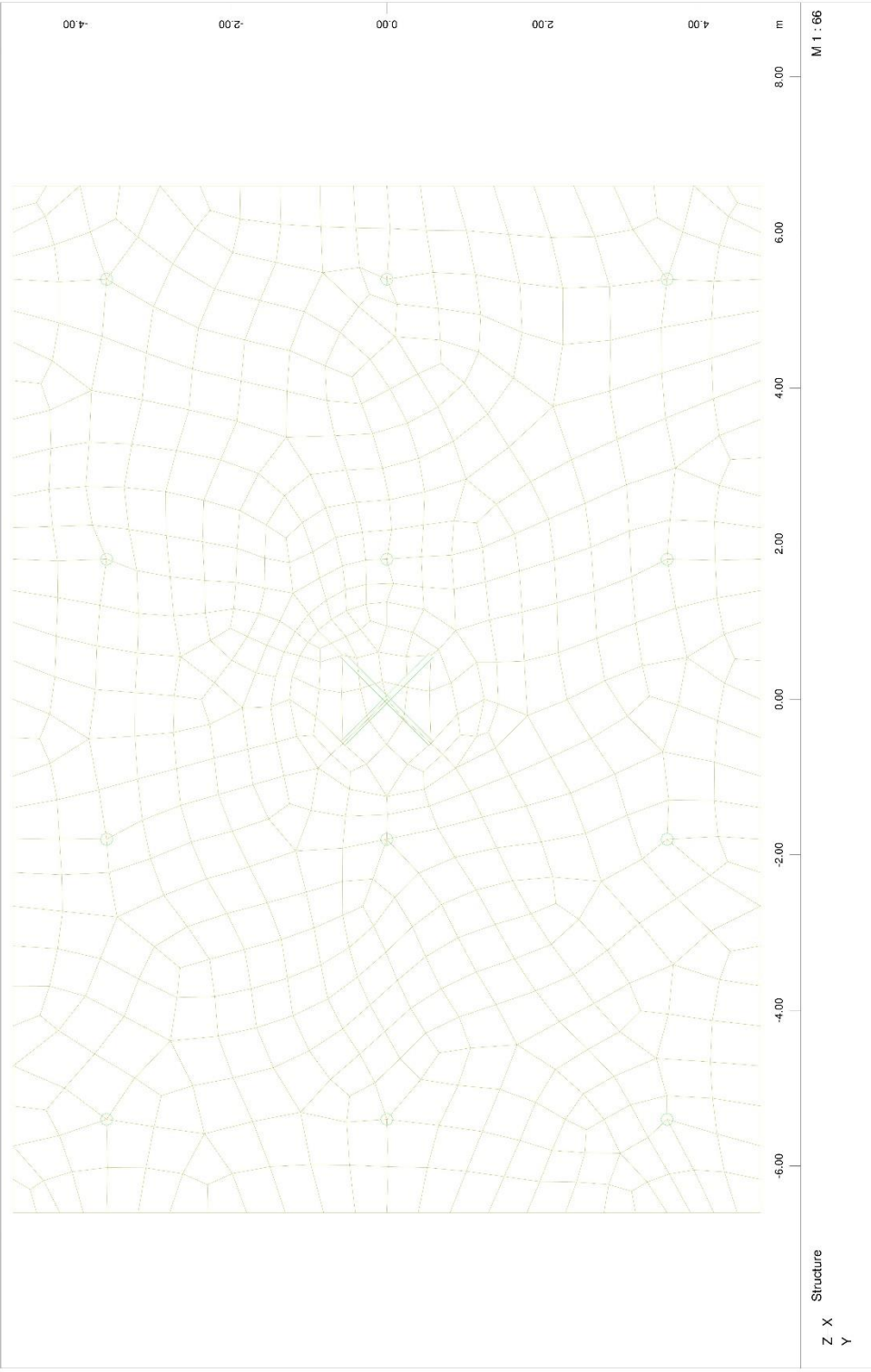
FOUNDATION OF PIER M5.A - STRUCTURE 7 PILE CAP FINITE ELEMENT MESH
