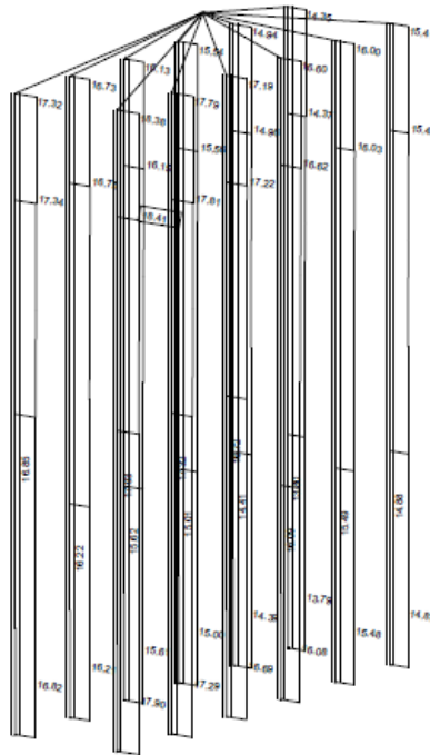
Beam Elements , Longitudinal Reinforcements Lay. 1, Design Case 1 , 1 cm 3D = 50.0 cm2 (Max=18.4)
