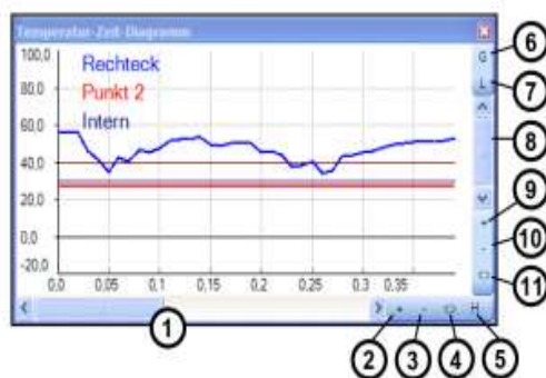
Control elements of the time axis
