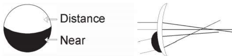
Figure 1 Diagram of an alternating vision RGP lens. The upper and lower parts of the lens provide distant and near vision, respectively.
