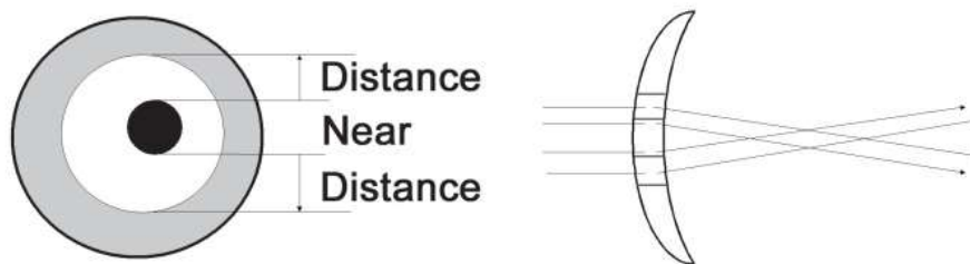
Figure 4 Diagram of a lens in which the optical axis coincides with the line of sight. In this design, the optical center of the lens is shifted slightly toward the nose so that it coincides with the line of sight. Since convergence and miosis occur at the time of near vision, this design is most suitable for near vision.
