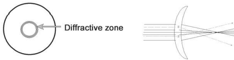
Figure 5 Diffractive SCL. There is a refractive part at the center, which is surrounded by many circular diffractive zones. A distant image is formed by refraction at the center, while a near image is formed in the diffractive zone on the inner surface of the lens.
