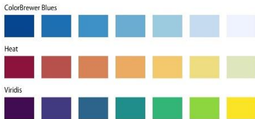
Figure 4-3. Example sequential color scales. The ColorBrewer Blues scale is a monochromatic scale that varies from dark to light blue. The Heat and Viridis scales are multihue scales that vary from dark red to light yellow and from dark blue via green to light yellow, respectively.
