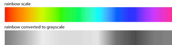
Figure 19-4. The rainbow color scale is highly nonmonotonic. This becomes apparent when the colors are converted to gray values. From left to right, the scale goes from moderately dark to light to very dark and back to moderately dark. In addition, the changes in lightness are nonuniform. The lightest part of the scale (corresponding to the colors yellow, light green, and cyan) takes up almost a third of the entire scale, while the darkest part (corresponding to dark blue) is concentrated in a narrow region of the scale.
